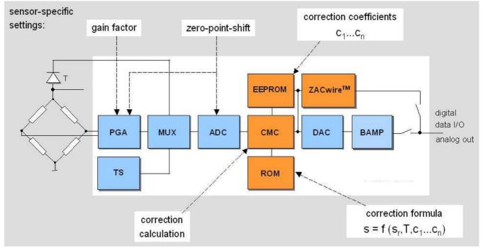
Fig.2: Block diagram of ZMD31150
