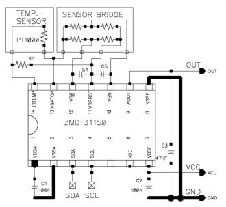
**Example 2**: Bridge in voltage mode, external thermistor
